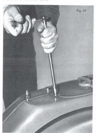
Fig. 36 - Dismantling of the unit petrol (gas) tank-oil tank: Act as shown in figs. 33 and 34 for lifting the fuel tank-oil tank unit.
